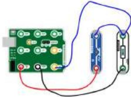
For the light level received by the sensor, you will have to convert this magnitude into a numerical value. To do this, you must use the communications built into the Cirkids microcontroller module.
