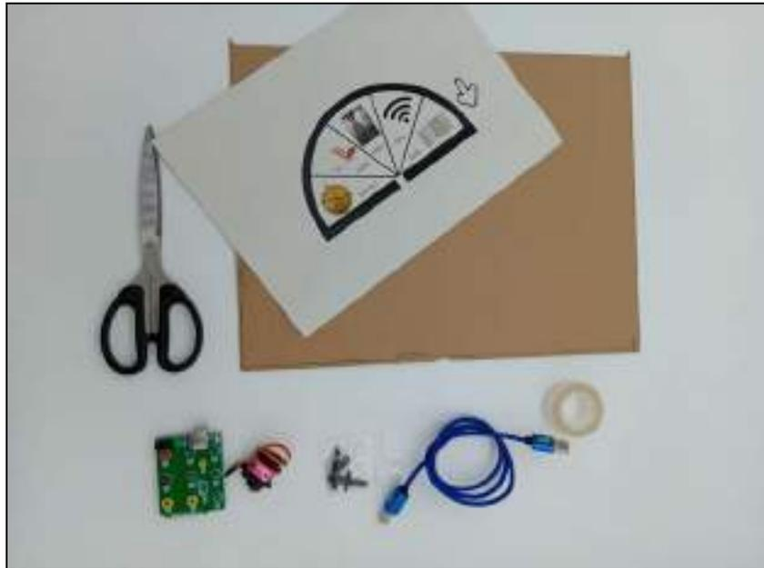
Glue the timeline onto the cardboard and cut it to shape - remember to leave a hole for the servo motor!
