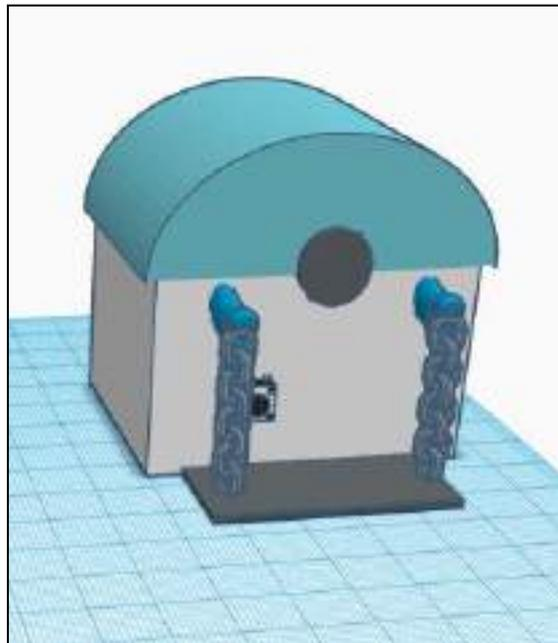
Sometimes, the hole to put the rubbish in the containers is too high. For this reason, this model has a platform that goes up when you press the button.
