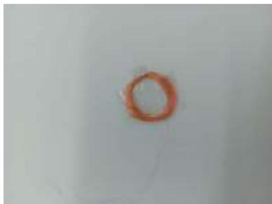
Once you have created the coil, make sure to leave at least 3 cm of copper at the ends so that you can connect the wires to the microcontroller. To make the electrical connection, you will need to remove the enamel (insulation) from the copper coil. You can use scissors, sandpaper or even a lighter to do this.
