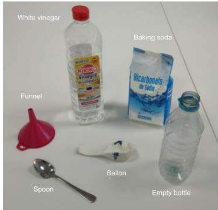
Approximately 20 ml of vinegar is poured into the bottle, and then about 5 grams of baking soda (one tablespoon) is added, and we wait for the reaction to occur. Once our balloon is well inflated, we bend it a little at the base before removing it to keep it closed (but not tied) to prevent the carbon dioxide we generated from escaping. We will keep it pinched with our fingers at the opening, as shown in the image, to prevent the gas from escaping while we transfer it to another container.
