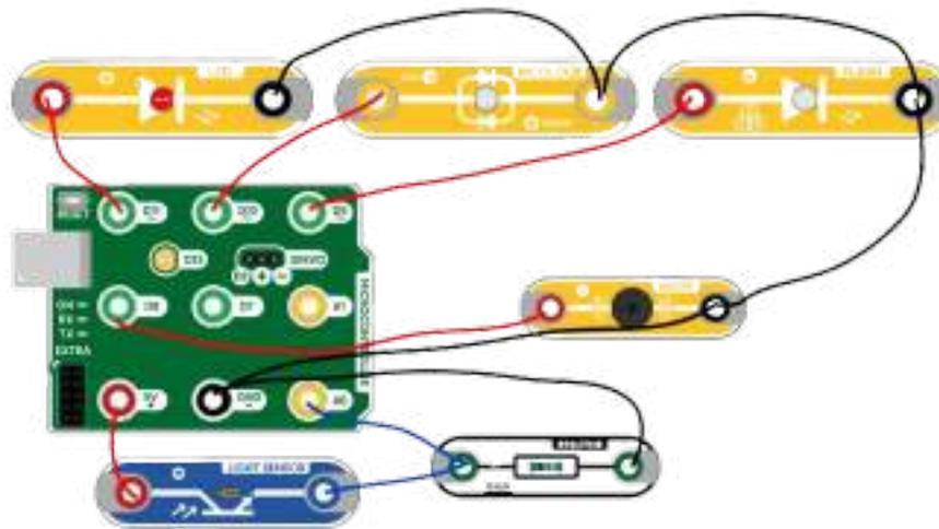
One of the possible errors that can occur when working with this block for the first time is not updating the pin of the component. In this case, the buzzer has been connected to digital pin 8, so it must be updated in the drop-down menu. The negative pole of the buzzer has been connected in series to the LEDs. On the other hand, you can also choose the song of your choice from those available in the drop-down menu.
