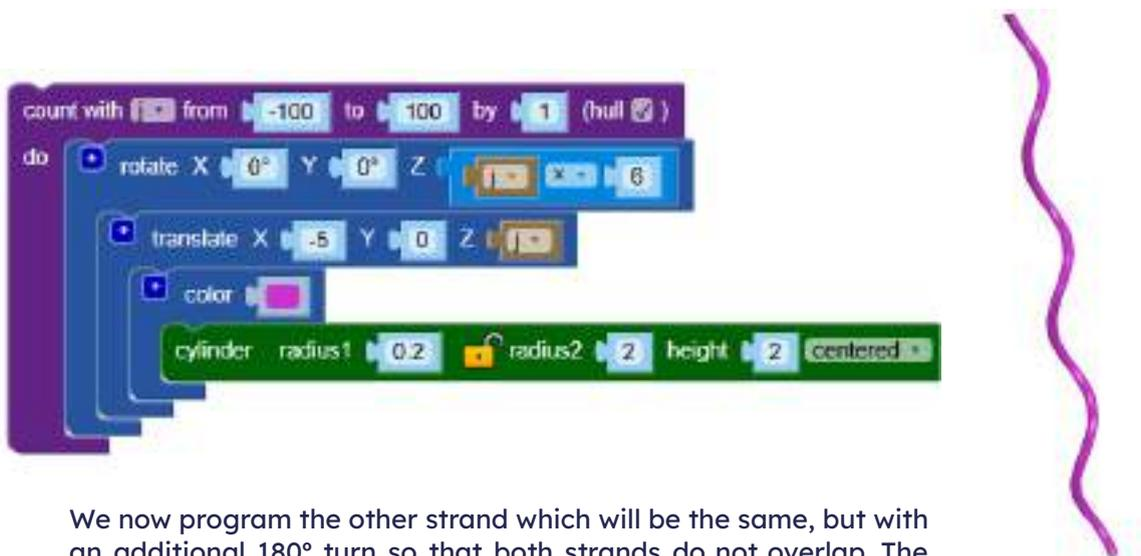
We now program the other strand which will be the same, but with an additional 180° turn so that both strands do not overlap. The turn must be programmed on the Z axis.
