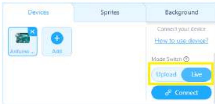
In order to be able to interact with the elements on the screen, the device must be connected in 'live mode' and once you have made sure of this, click 'connect'.
