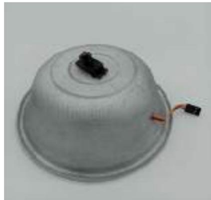
On the front, place the button with the red LED. The button will be in charge of starting the activity. When it is pressed, the robot will begin to analyze our command. The red LED indicates when the robot is listening.
