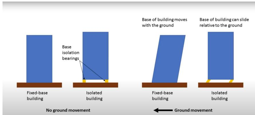
One way of counteracting horizontal seismic forces in the ground is, on the one hand, to place the foundations of a building above the surface level and, on the other hand, to separate them from the subsoil with the help of elastic rubber bases composed of layers of steel, rubber and lead. When the subsoil moves during the earthquake, the anti-seismic supports vibrate next to it and absorb most of the kinetic energy, affecting the building less, in a similar way to the shock absorbers of a car.
