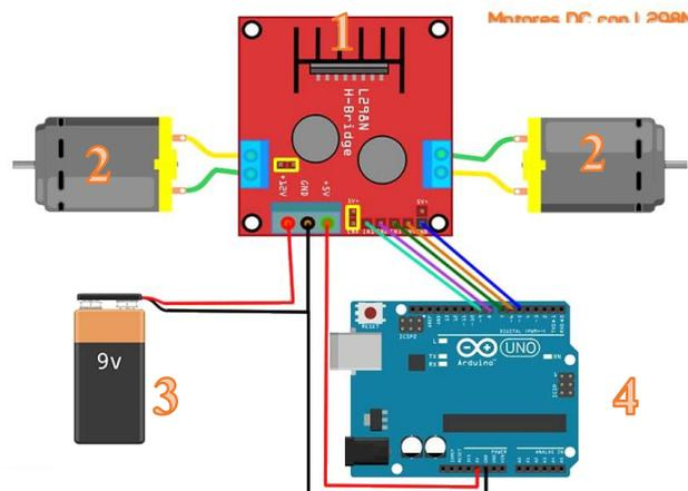
This is a basic diagram for connecting DC motors to the L298N motor driver using an Arduino board and a power source. Here's a step-by-step explanation of the setup:
