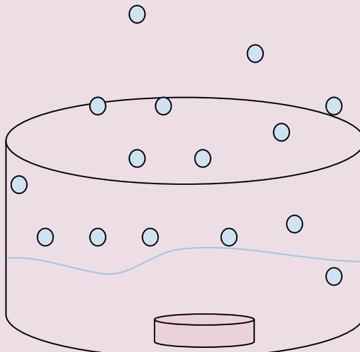
On the other hand, for our rocket, as it is covered (not open), all those CO<sub>2</sub> molecules that combine with the air, instead of being released into the atmosphere, start to accumulate inside the covered cylinder that we have prepared. There comes a point when the pressure inside the cylinder is so high, due to the amount of gas accumulated, that the same pressure causes the lid to fly off, as it is not sealed but a movable lid.
